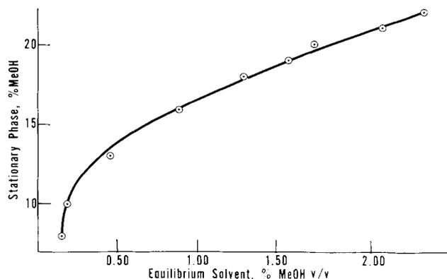
FIG. 2. Methanol concentrations of equilibrated solvents from slurries of methanol-benzene silicic acid.
