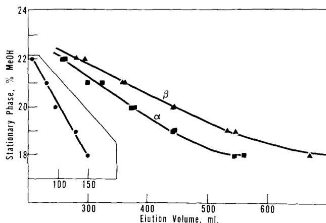
Fig. 6. Effects of different concentrations of stationary phase methanol on elution volumes of  $\alpha$ - and  $\beta$ -monoglycerides of soybean oil. Insert: Peak separation between  $\alpha$ - and  $\beta$ -monoglycerides of soybean oil.
