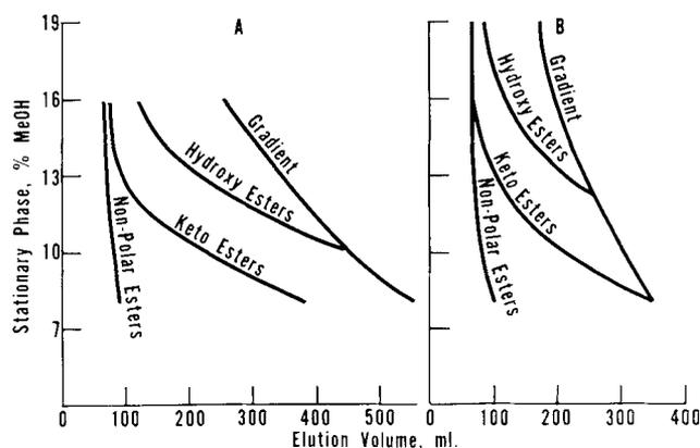
FIG. 4. Effects of different concentrations of stationary phase methanol on elution volumes of nonpolar, keto and hydroxy fatty acid methyl esters and on the gradient. Mobile solvent: A, 1% methanol in benzene by volume. B, 2% methanol in benzene by volume.
