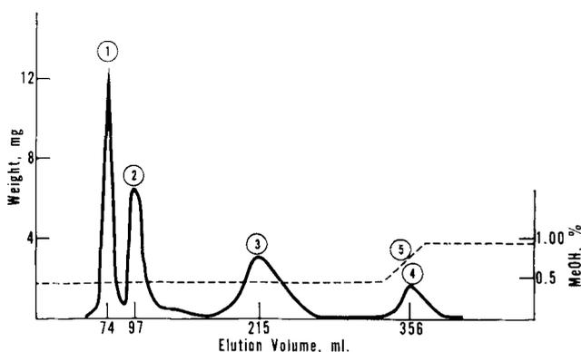
FIG. 3. Chromatographic separation of a fatty acid ester mixture: 1, nonpolar; 2, keto; 3, hydroxy; 4, oxidation products and 5, gradient. Mobile solvent: 1% methanol in benzene by volume. Stationary phase: 13% MeOH to  $\text{SiO}_2$  by weight.
