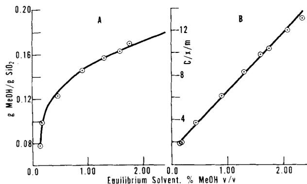
FIG. 1. A, adsorption isotherm for methanol on silicic acid. B, a plot of Langmuir's equation,  $c/x/m = 1/a + \beta c/a$ ,  $c =$  conc. of MeOH in solution,  $x/m =$  g MeOH adsorbed.
