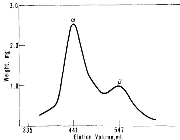
FIG. 5. Chromatographic separation of  $\alpha$ - and  $\beta$ -monoglycerides of soybean oil. Mobile solvent: 1.6% methanol in benzene by volume. Stationary phase: 19% MeOH to  $\text{SiO}_2$  by weight.
